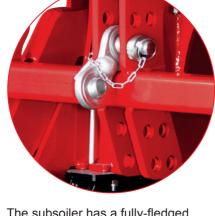
The subsoiler has a fully-fledged, parallel-guided linkage with integrated upper linkage point. This allows the working depth of the subsoiler compared to the follow-up device to be adjusted hydraulically during work. Due to the specially developed hydraulic three-point linkage the entire implement combination is only extended by only approx. 85 cm when driving on the road.
